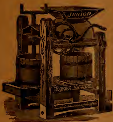
Cider Mills—with wooden crushing rollers.
